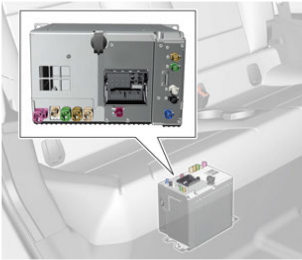
Installation location of Headunit High in the I01
